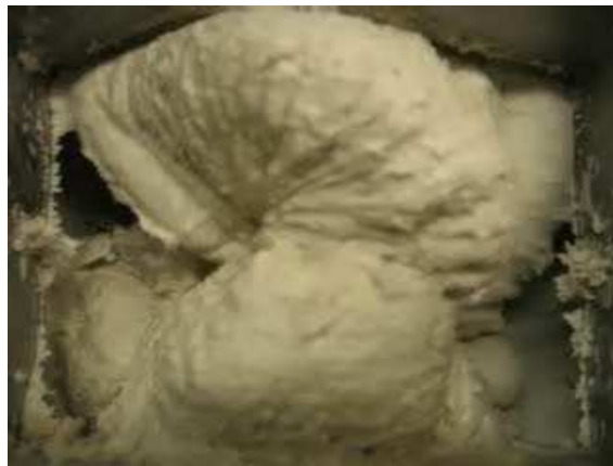
Fig.4: Bridging in the Farinograph ® wheat mixer while testing milled rye products.
